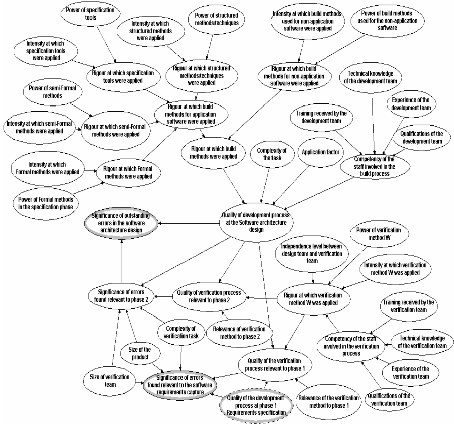
Fig. 5. Hugin screenshot of the process model for the ‘Software Architecture Design’ phase of the IEC61508 software development lifecycle
